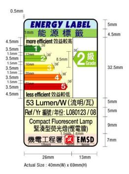
(3) The energy label under clause 1 of Appendix 3B is divided into 3 rectangular areas (marked I, II and III by the side of the label). The information to be contained in each area of the energy label is specified in column 2 of the following Table in relation to the area specified opposite to that information in column 1 of the Table.
