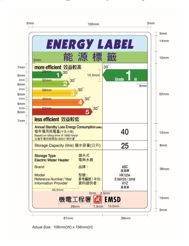
(3) The energy label under clause 1 of Appendix 7B is divided into 4 rectangular areas (marked I, II, III and IV by the side of the label). The information to be contained in each area of the energy label is specified in column 2 of the following Table in relation to the area specified opposite to that information in column 1 of the Table.
