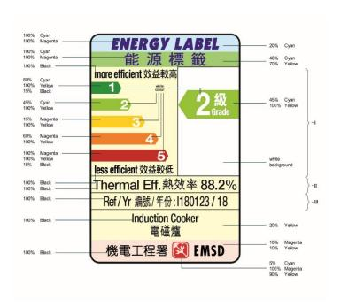
(2) The dimensions of the energy label must be as specified in the diagram below—
