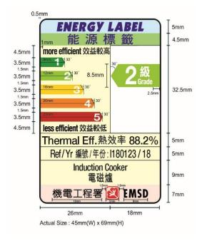
(3) The energy label under clause 1 of Appendix 8B is divided into 3 rectangular areas (marked I, II and III by the side of the label). The information to be contained in each area of the energy label is specified in column 2 of the following Table in relation to the area specified opposite to that information in column 1 of the Table.
