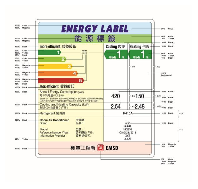
(3B) The dimenisons of the energy label for a room air conditioner of reverse cycle type must be as specified in the diagram below—
