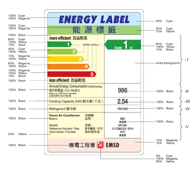
(2) The dimensions of the energy label for a room air conditioner of cooling only type must be as specified in the diagram below—
